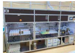
Automated specimen processing device for measuring the quantity of the active ingredient in our ONPO product
